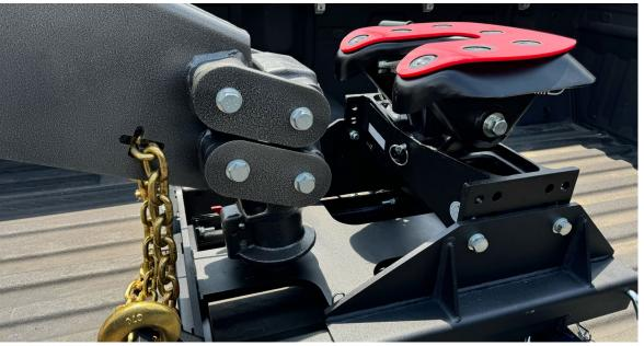
5TH WHEEL & GOOSENECK COMBO HITCH TOWING 25,000 LBS. TONGUE WEIGHT 6,000 LBS.
